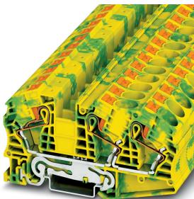
Ground modular terminal block, number of connections: 3, connection method: Push-in connection, 1 level, Rated cross section: 16 mm<sup>2</sup>, cross section: 0.5 mm<sup>2</sup> - 25 mm<sup>2</sup>, mounting type: NS 35/7,5, NS 35/15, color: green-yellow
