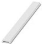
Zack Marker strip, flat, can be ordered: Strip, white, labeled according to customer specifications, mounting type: snap into flat marker groove, for terminal block width: 12 mm, lettering field size: 5.15 x 12.15 mm, Number of individual labels: 5
